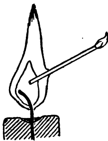
Fig. 29.—Conducting gases from dark zone.
